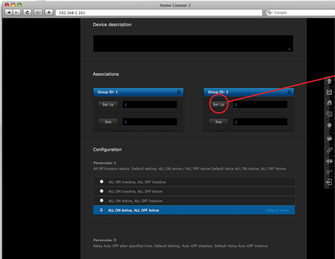
Now click "Set up" button corresponding to chosen association group. Fibaro Relay Switch 2x1,5kW supports two, independent association groups: ID1 and ID2, triggered by key 1 or key 2 of the switch, respectively.
