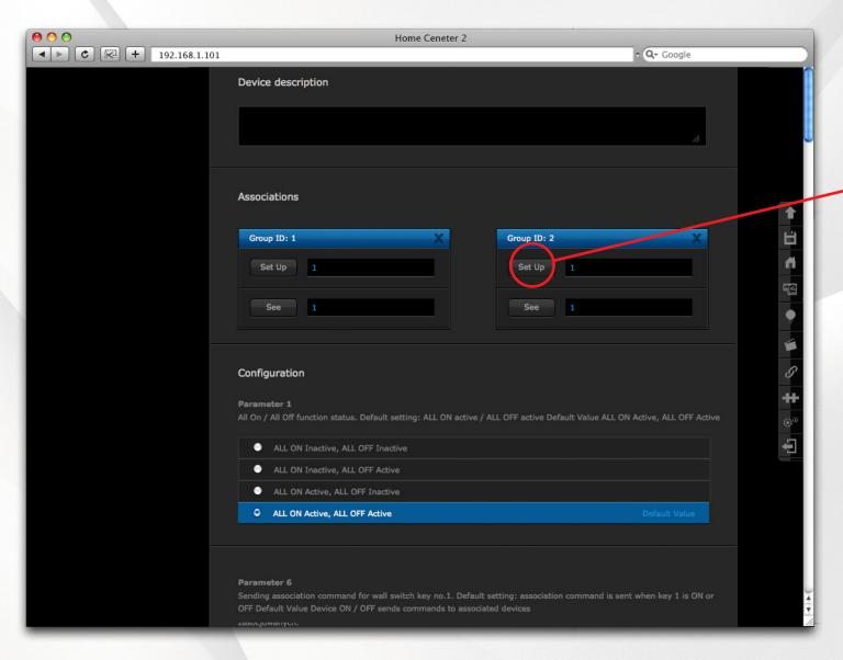
Now click "Set up" button corresponding to chosen association group. Fibaro Dimmer supports two, independent association groups: ID1 and ID2, triggered by key 1 and key 2 of the wall switch, respectively.
